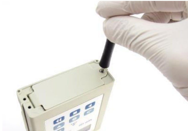
Figure 7: Open the battery compartment with a T10 Torx key.
