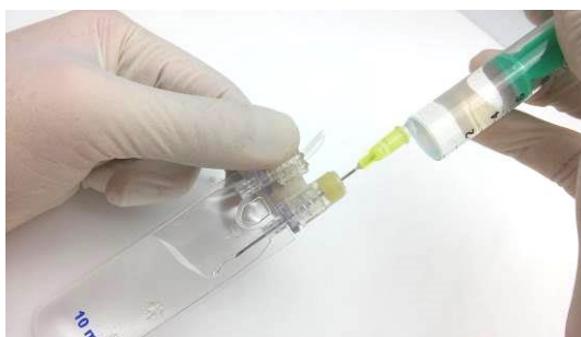
Figure 13: Filling the perfusate bag via injection port
