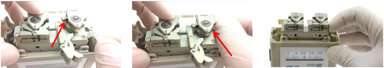
Figure 15: Inserting the tubing into the pump module
